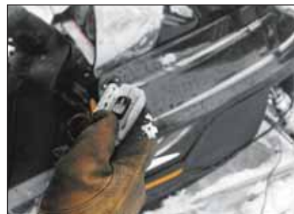
Hand-held remote control with 12-1/2' lead for full range of movement during winching
