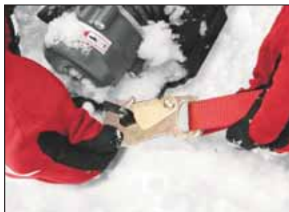
Hooks and mounting plate connect winch to the sled
